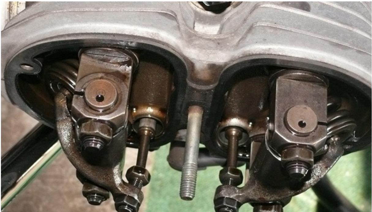
Re-tension the head nut to the nominated specifications, set the valve clearance, replace the oil filter (*remembering to check the proverbial '\$2,000 O ring' clearance*) refill the oil, close it up and it's time to test.
