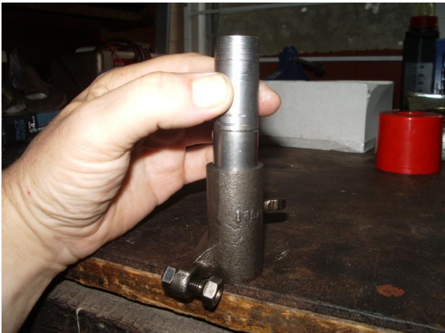
Use either a press or a vice to push the bearings into place. ***(Nb: Do not use a hammer against the pressing tool, or the bearing to tap it into place. The outer cage of needle rollers are easily damaged.)***
