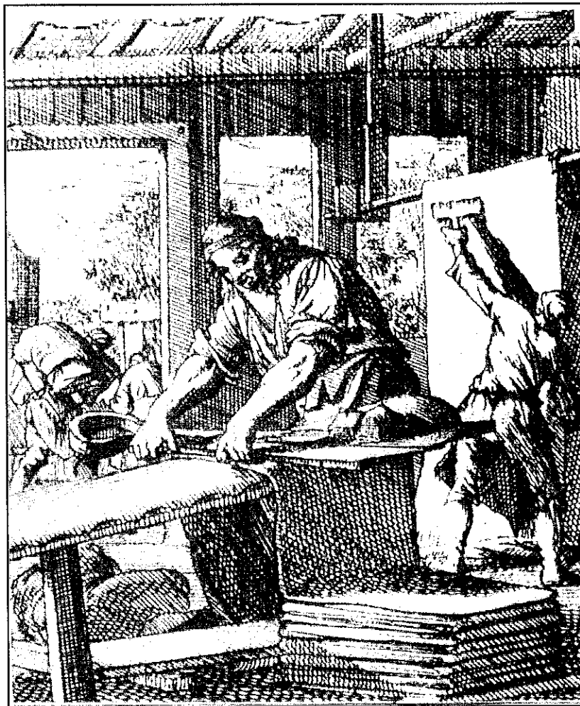
A reproduction of a 17th century engraving showing "teasing" and shearing of broadcloth by hand.
